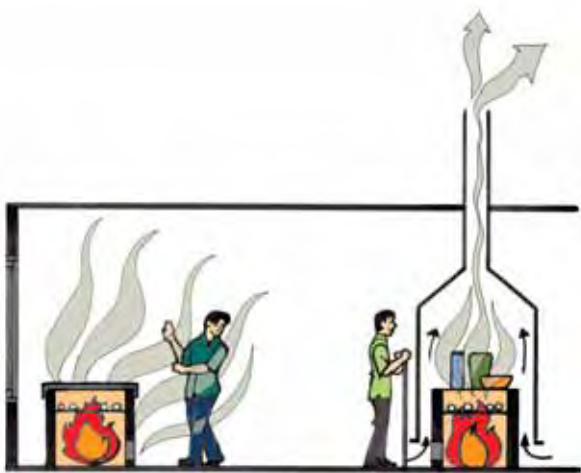
Figure 50: Use local exhaust ventilation against heat radiation and pollution.
