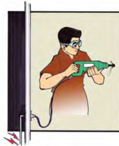
Figure 28: All electrical equipment should be earthed correctly. An independent earthing rod should be used to connect earthing wires from machines.
