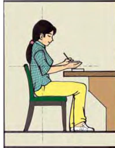
Figure 31: Provide seated workers with chairs of correct height with sturdy backrest, with the feet comfortably placed on the floor.
