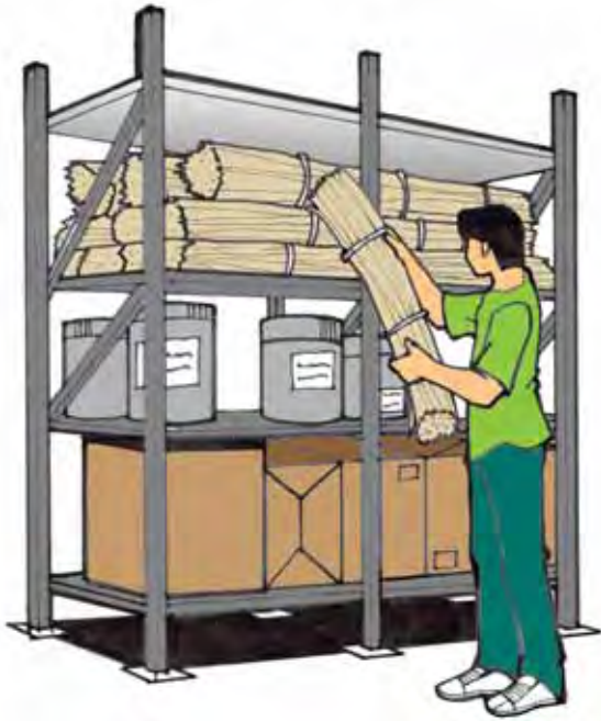
Figure 7: Multi-level rack for storing materials, tools, and products.
