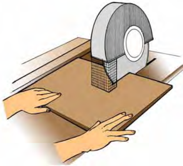
Figure 16: Attach proper guards to dangerous moving parts of machines such as exposed gears, chain drives and projecting shafts.
