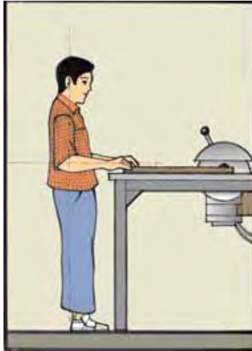
Figure 30: A working height at elbow level or slightly lower than elbow level minimizes muscular effort.
