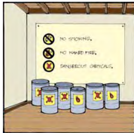
Figure 51: Store hazardous chemicals outside work areas with a firm lock. Ensure children do not come into contact with them.
